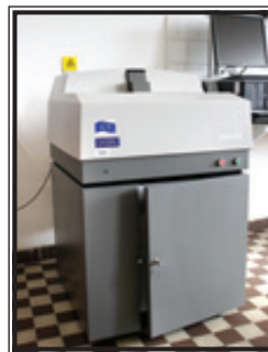
WDXRF- for analysis of sulphure in the oil derivatives
